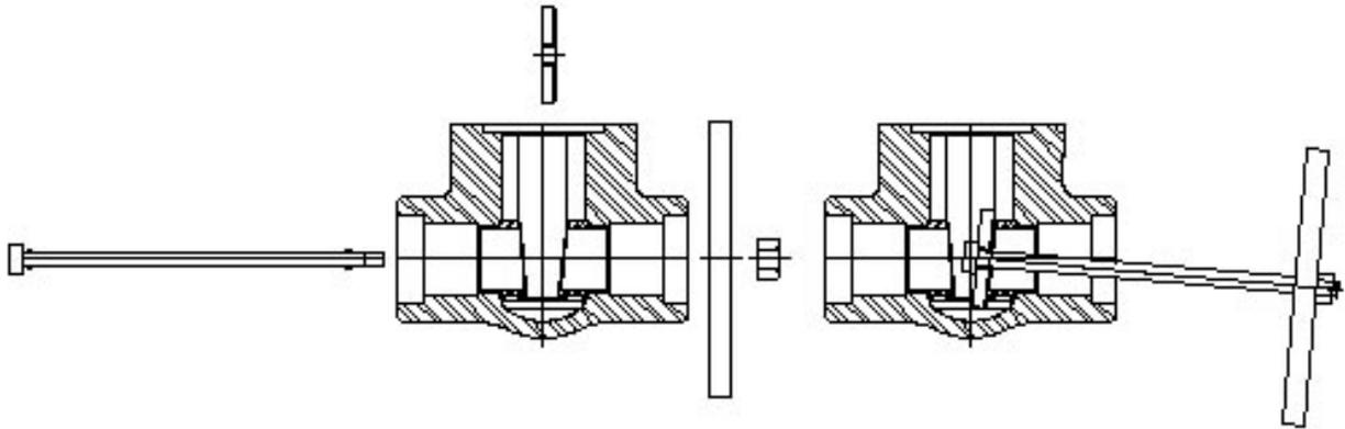
**FIGURE 5: Seat Rings Lapping**
