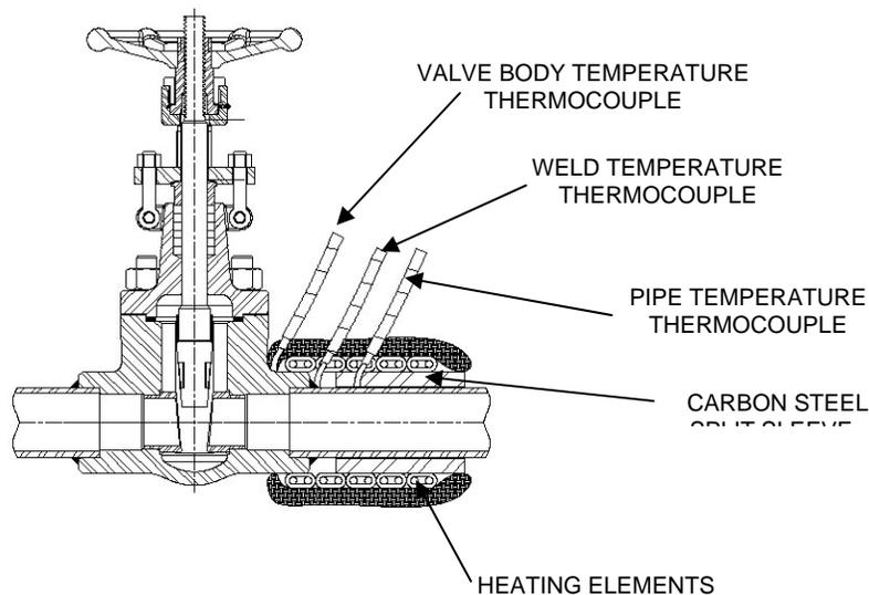
**FIGURE 4: Typical Post Weld Heat Treat Arrangement**
