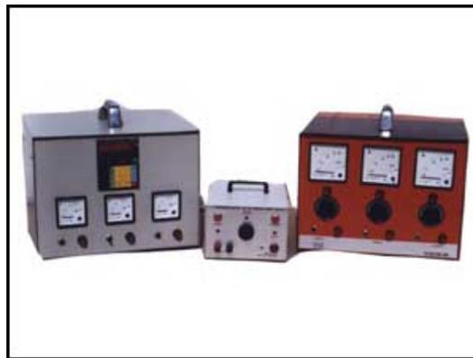
**FIGURE 2 Multi Outlet Power Transformers and Controller for PWHT**
